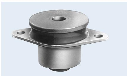
500 Series mounts are low cost isolators that provide high load carrying capacity, compact size and stability. These all attitude mounts are perfect for isolating truck, bus and marine engines.
